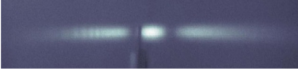
Figure 5. Image of the laser diode on its mount and the far field projected onto a screen.
